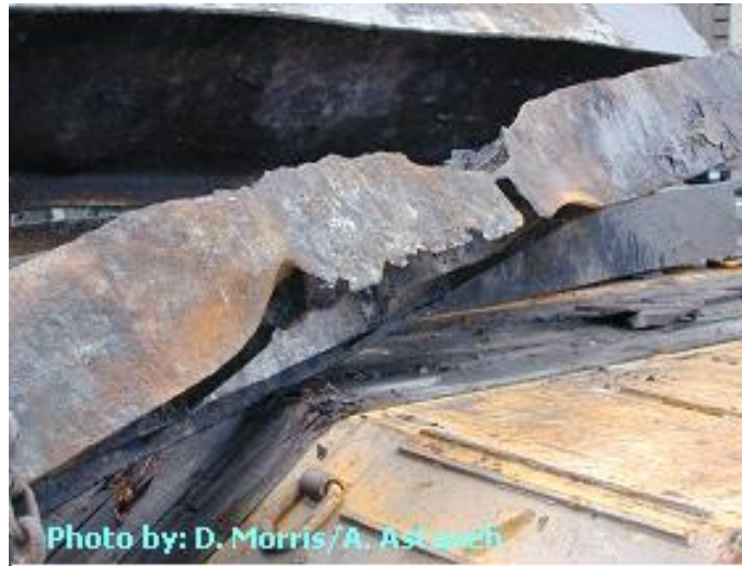
Figure 10. A Beam Removed From the World Trade Center the Site Most Probably From Building 7 (Ref: Astaneh-Asl, 2002b)
